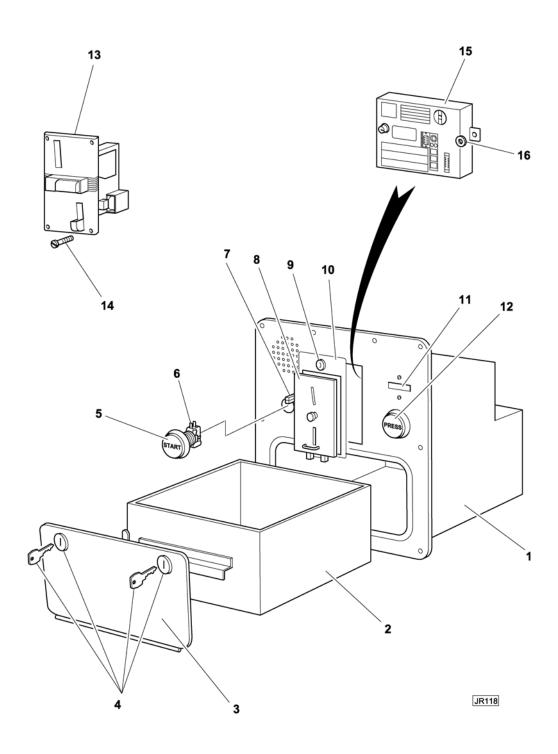
Fig 6 Coin collection assembly (System 4000)
